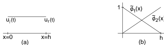
Figure 8.9. (a) Rod displacements u_\ell(t) and u_r(t) at the left and right endpoints of the local interval [0, h] . (b) Local linear basis functions \tilde{\phi}_1(x) and \tilde{\phi}_2(x) .
