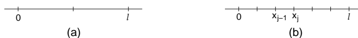
Figure 8.10. Partition of the rod domain [0, \ell] into (a) 2 subregions and (b) n subregions.
